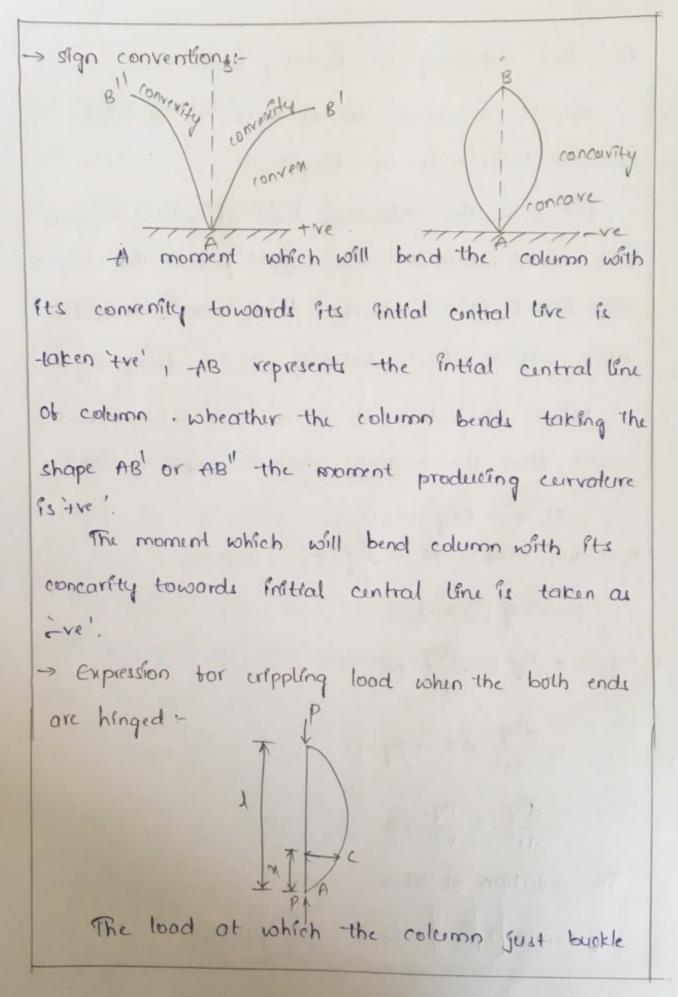
is called creppling or ) buckling load.
