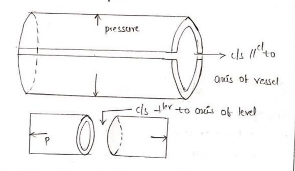
stresses in a thin cylindrical vessel subjected to internal
