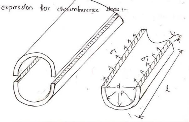
consider a thin cylindrical vissel subjected to internal fluid pressure the circumferential stress will be salup in the material of cylinder, It the brusting cylinder takes place, -continuation
