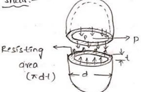
At then spherical shell of internal dia d'andthiekn —ess il and subjected to an internal fluid pressure p'
