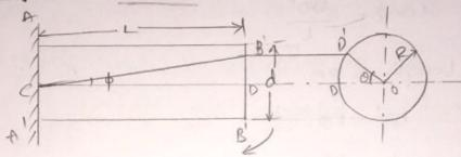
shaft is fixed at one end and torque being applied on the other end.
