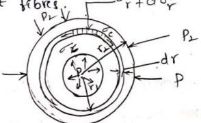
consider a thick cylinder subjected to internal and external stress (pressure).
