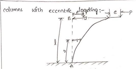
A column AB of length 'I' fixed at one end B' and free at 'A'. A column is subjected to load b' which is an eccentric by amount of 'e'. The free end swaly side ways by amount of 'a' and the column will diffect.
