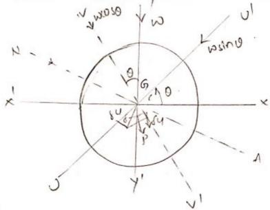
A transverse section of bram with centroid is? along with rectangular co-ordinate axis x-x and y-y!. The principal axis uvi and vvi inclined at an angle of to xy set of co-ordinate axis. wis the load acting along with the line y-y!. This load can be resolved into two components.
