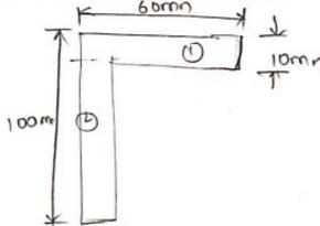
Dragram shows an unequal angle of dimensions 100mm x 60mm and 10mm thick. Determine.
