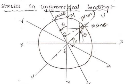
The clan of a beam subjected to B.M of m' for the plane of y-y. The co-ordinate axis' x-x 4 y-y pass through the centroid 'of' of the section. Let uv, vv are the principal axis passes through 'c' and forced at angle o' to xx and yy axis respectively
