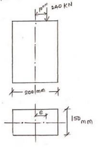
For the above problem min. stress on the section is given o. Then find eccentricity of the point load 240 KN acting on the rectangular column also calculate the corresponding max. stress on the section.
