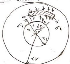
A spherical shell is subjected to internal pressure p'
