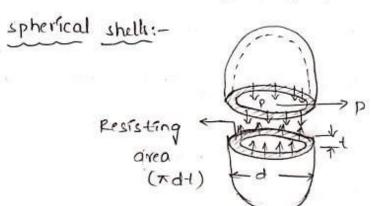
A then spherical shell of internal dia d'andthiekn -ess il and subjected to an internal fluid pressure p' - the fluid inside the shell has a tendency of splitte into hery spheres along x-x axis.
