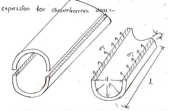
consider a thin cylindrical vessel subjected to internal fluid pressure the circumferential stress will be setup in the material of cylinder, If the brusting cylinder takes place, -continuation.
