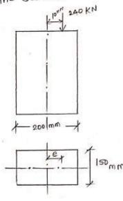
For the above problem min. stress on the section is given o. Then find eccentricity of the point load 240 KN acting on the rectangular column also calculate the corresponding max. stress on the section.
