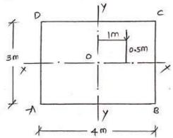
$$\sigma_{\text{max}} = \frac{80}{3\times4} - \frac{80\times1\times2}{16} - \frac{80\times0.5\times3/2}{9} = -10 \,\text{KN/m}^2$$
