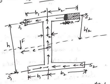
The unequal e-section. It is symmetrical bout x-x axis. hence shear center will lie on this axis.
