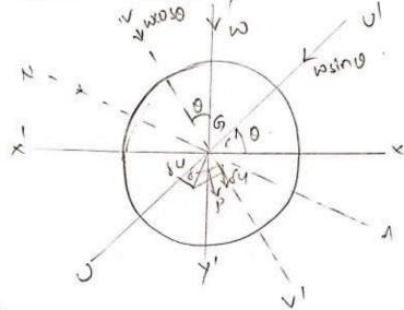
A transverse section of bram with centroid is? along with vectangular co-ordinate axis x-x and y-y!. The principal axis uvi and vvi inclined at an angle of to xy set of co-ordinate axis. wis the load acting along with the line y-y!. This load can be resolved into two components.
