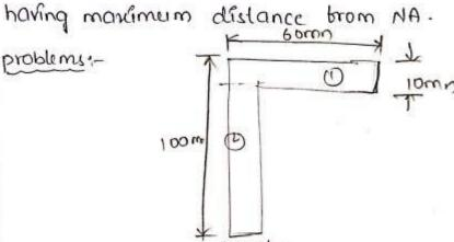
. Dlagram shows an unequal angle of dimensions 100mm x 60mm and 10mm thick. Determine.
