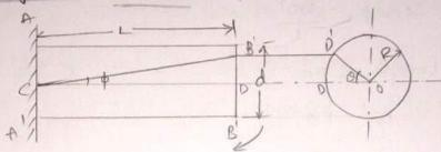
shaft is fixed at one end and torque being applied on the other end.
