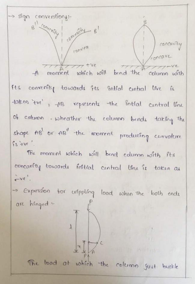
is called creppling or buckling load.
