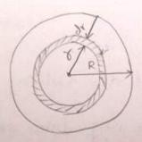
Maximum torque transmitted by a circular solid shaft is obtained from the maximum shear stress induced at the outer surface of the solid shaft.
