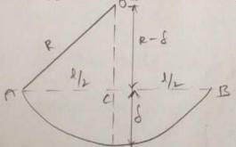
R - Radicus of the plate to which they are bent from Laco =  $0/4^2$ =  $Aot = Ac^2 + oc^2$
