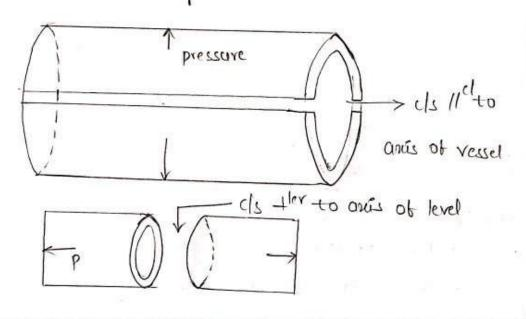
stresses in a thin cylendrical vessel subjected to internal
