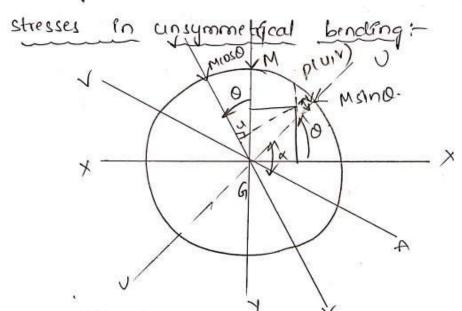
The clan of a beam subjected to B.M of m' for the plane of y-y. The co-ordinate axis' x-x 4 y-y pass through the centroid 'of of the section. Let uv, vv are the principal axis passes through 'c' and inclined at angle o' to xx and yy axis respectively
