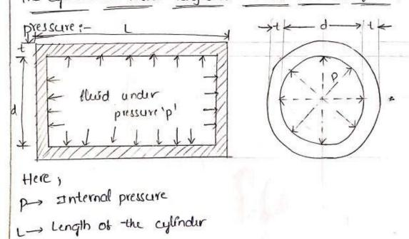
$d \rightarrow$  Internal da of the cylinder  $t \rightarrow$  thickness u 11 11
