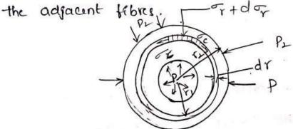
consider a thick cylinder subjected to internal and external stress (pressure).
