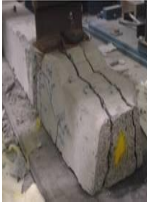
Fig. 2 Load induced deterioration
