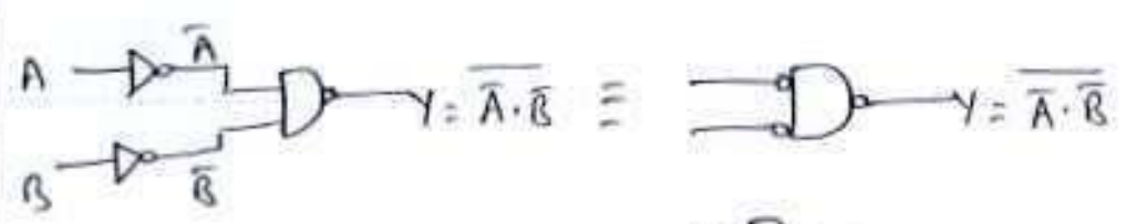
fig : AND function using NAND gates.
